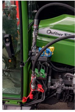
The hydraulic comfort connection only requires a pressure connec- tion and a pressure-free return. There are no extras controllers required.
